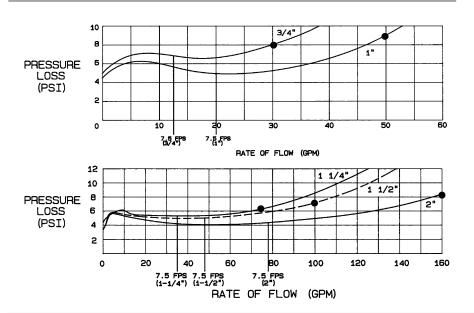
(•) Rated flow as determined by USC's FCCC & HR and ASSE design performance standards.
