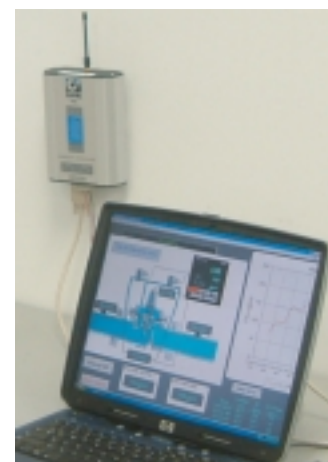
VSC Base Station & V-SCADA software
