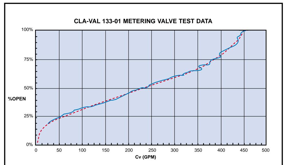
This Graph represents a compilation of test data used to evaluate the accuracy of the Cla-Val Model 133-01 Electronic Metering Valve. The dotted line shows the flow curve (Cv vs. %Open) that is characteristic of the valve. The solid line indicates the actual flow curve from tests. The test data was taken from a calibrated magnetic meter at varying flows, pressure differentials and valve positions and plotted against the valve characteristic curve for comparison.
