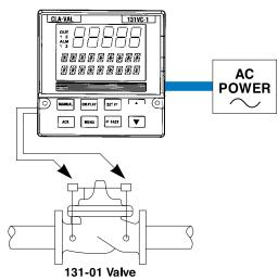
Maintain Valve Position When there is a power failure, using the standard Model 131-01 Control Valve, the pilot control solenoids lock in the closed position and hold the main valve in the last control position.
