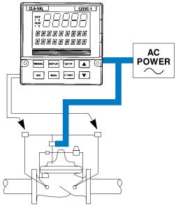
Hydraulic Backup A second hydraulic pilot system is arranged in parallel with the electronic system. On power failure, a third solenoid switches the control from electronic to the backup hydraulic system. The hydraulic system will then modulate the valve to maintain preset system conditions. Virtually any hydraulic system can be used (we have many to fill your application requirements).
