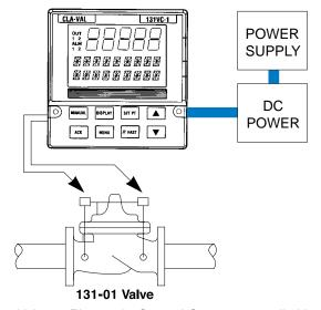
Direct Voltage Electronic Control Customer supplied battery power with a continuous charging system operate the valve solenoids and controller in the event of power failure.
