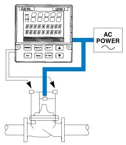
Open or Close Valve Adds a third solenoid control to the pilot system which either opens or closes the main valve on power failure.
