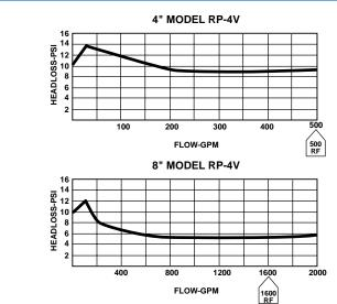
FLOW-GPM 1000 RF "Rated Flow" Values adopted by the American Water Works Association and the New England Water Works Association. 4" Model RP-4V Flow curve generated by the Foundation for Cross-Connection Control and Hydraulic Research at the University of California.
