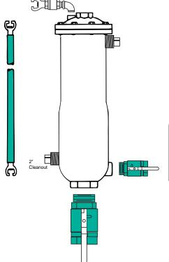
Series 35-WW with Optional Customer Installed BWKT Backwash Kit
