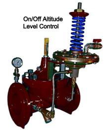
The CLA-VAL SERIES 210 On/Off Altitude Level Control Valve controls the high water level in a reservoir or closed tank without the need for floats or other devices. It is a non-throttling valve that remains fully open until the shut-off point is reached.
