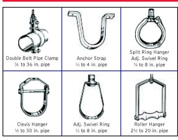
The pipe should not be anchored tightly by the support, but secured in a manner to allow for movement caused by thermal expansion and contraction. It is recommended that you use clamps or straps that allow pipe to remain away from the framing, thus reducing the noise generated when pipe is allowed to rub against wood.
