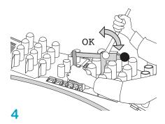
Start to fasten the ring around the pipe. Using the clamp, tighten each element up to the end of the third tooth.
