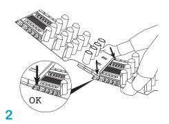
Insert the male button-strap into the slot of the next pieces until you have asembled the required number of elements to circle the pipe in order to create a belt of elements.
