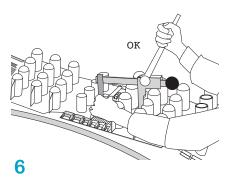
For the final clamping around the pipe, tighten gradually in order to obtain as much as possible an omogeneous number of engaged teeth.
