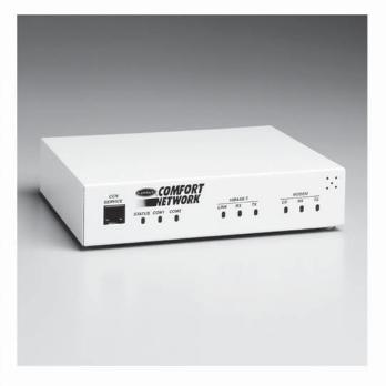
In this application each converter occupies a unique bus and element address on the CCN. When configured as a bridge, it is addressed similarly to other CCN Bridges where the system element number on the primary bus identifies the secondary bus number.
