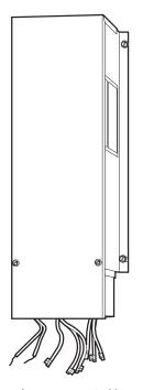
The Motormaster V head pressure control is used to permit low ambient operation down to -20~F by modulating the fan speed on each of the primary fans (1 and 2). The standard factory-installed motors are compatible with the Motormaster V control.
