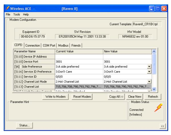
Check that the side preference is correct (step 11 in Airlink manual). To complete the configuration, proceed to step 13 in the AirLink manual (Write to Modem).
