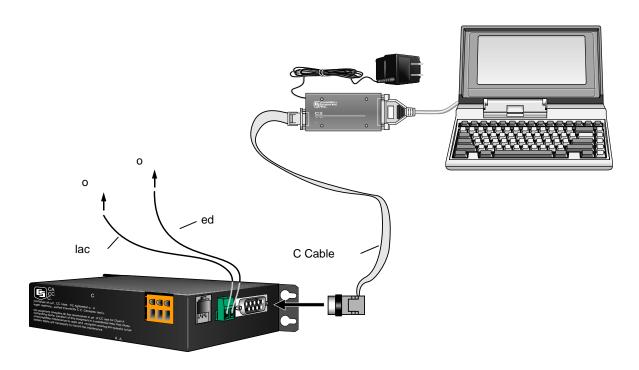
FIGURE A-1. COM200 to Computer Connection
