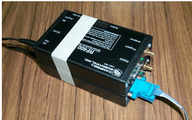
FIGURE K-1. Loop-back Test without Antennas
