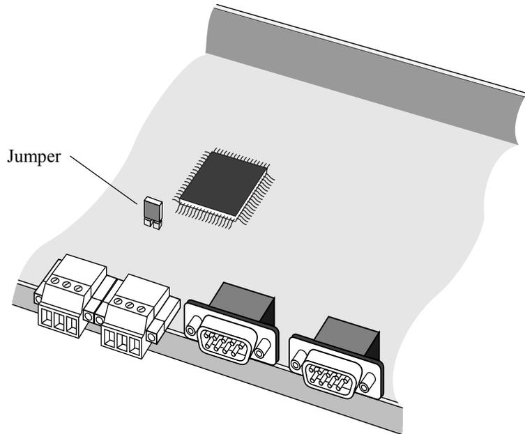
FIGURE 2. NL100/105 Jumper Placement
