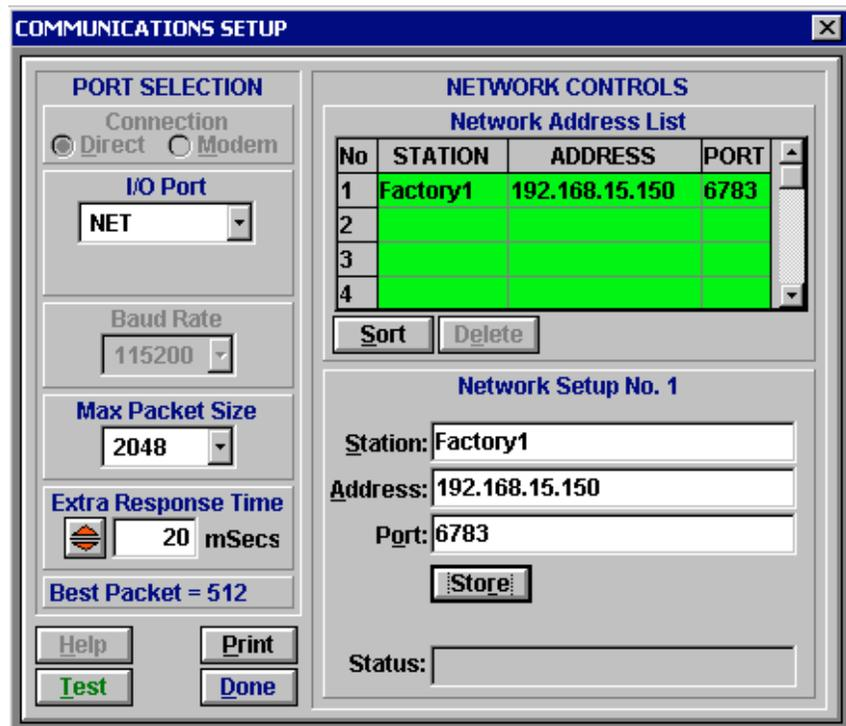
FIGURE 7. PC9000 Setup for TCP/IP Communication
