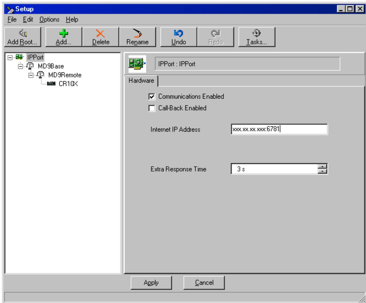
FIGURE 4. LoggerNet Setup for NL100/105 to MD9 to Datalogger Connection
