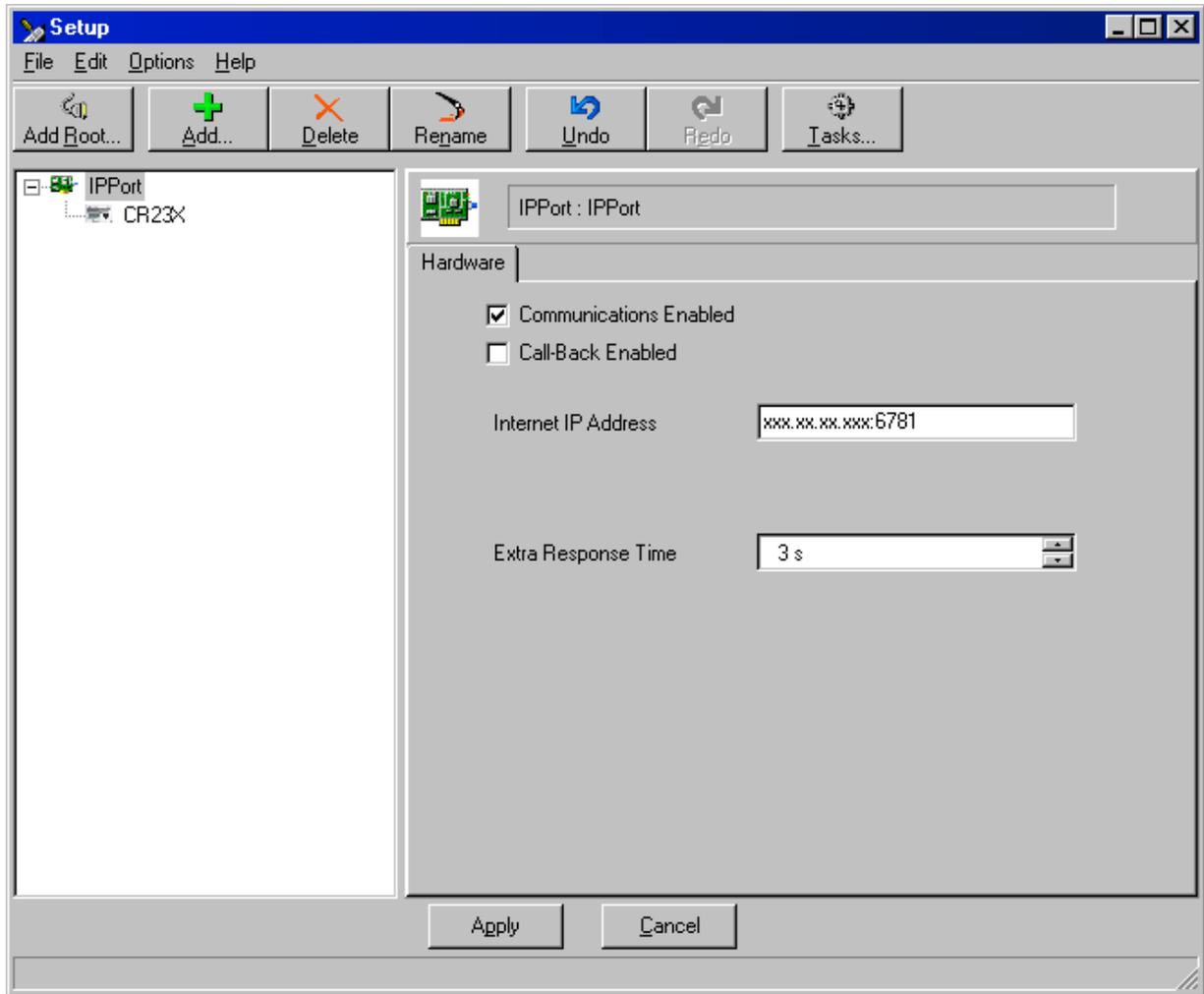
FIGURE 3. Typical NL100/105 Setup in LoggerNet
