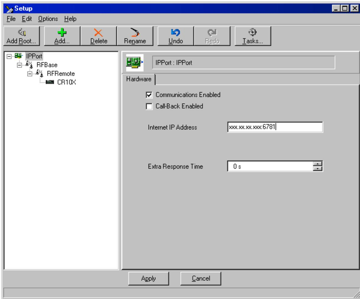
FIGURE 5. LoggerNet Setup for NL100/105 to RF to Datalogger Connection
