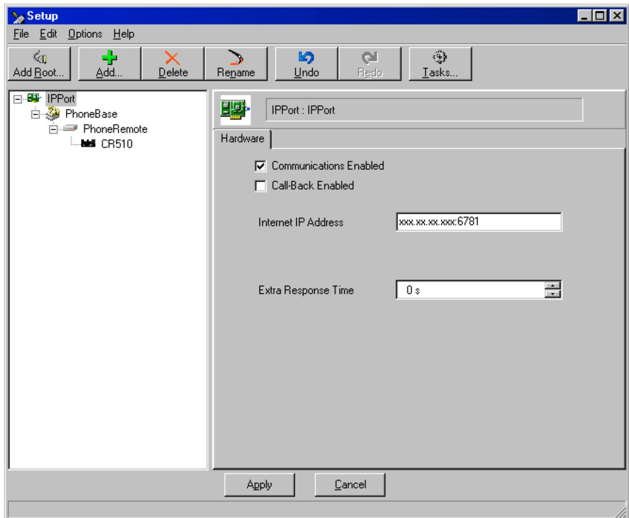
FIGURE 6. LoggerNet Setup for NL100/105 to Phone to Datalogger Connection
