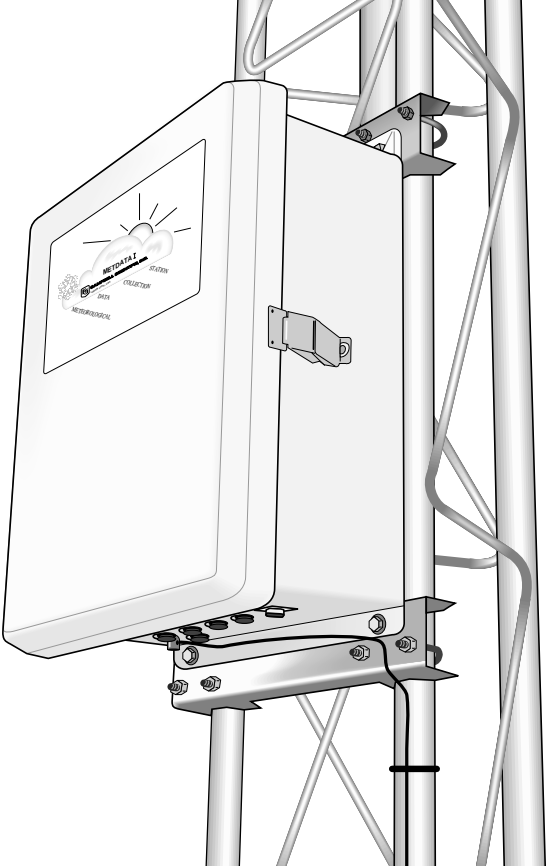
FIGURE 3.1-2. MetData1 Enclosure on UT10 or UT30 Tower
