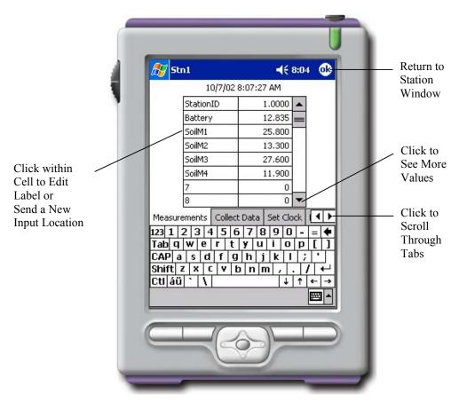
Because of the small screen size, you may see only a portion of the input locations in the datalogger. Touch the up or down arrows to the right of the measurement cells to scroll through the values.
