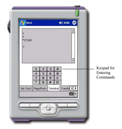
To return the datalogger to its program execution state, enter \*0. LOG1, LOG2, or LOG12 should be displayed indicating that the code in program table 1, and/or program table 2, is being run.
