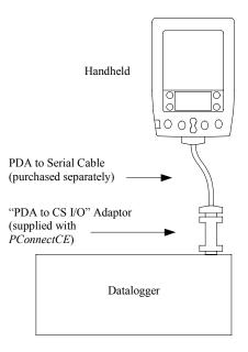
Note that one side of the connector is labeled Datalogger, and the other side is labeled PDA. If the connections are reversed, communication with the datalogger will fail.
