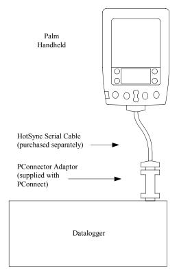
Note that one side of the connector is labeled Datalogger, and the other side is labeled PDA. If the connections are reversed, communication with the datalogger will fail.
