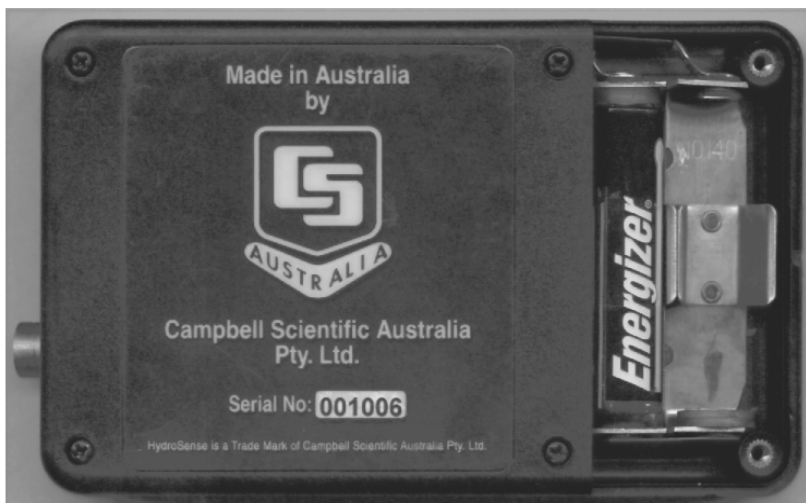
FIGURE 8-1. Rear view of the HydroSense display unit with battery cover removed
