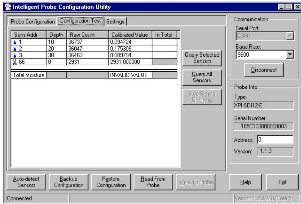
FIGURE B-7. IPConfig Configuration Test Window
