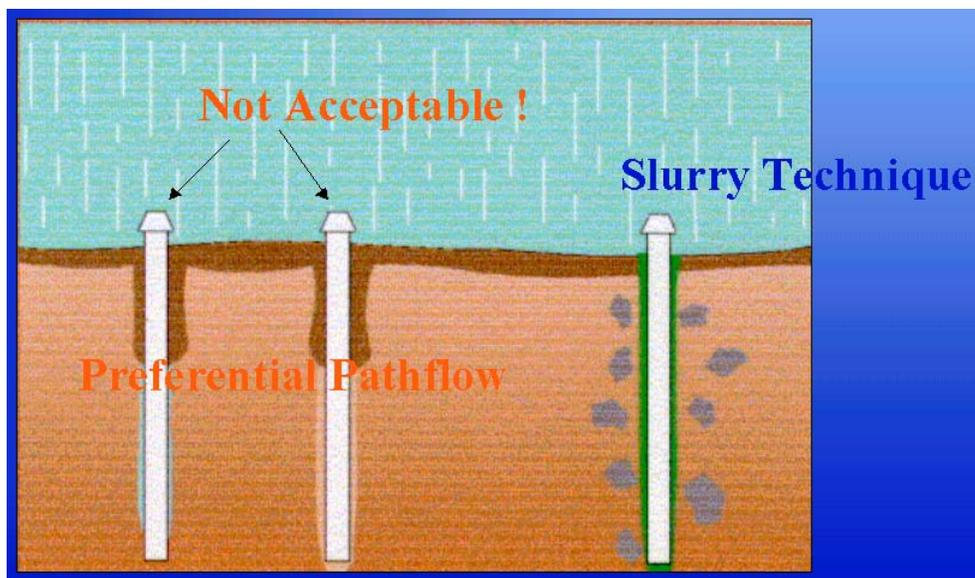
Figure C-1. Incorrect Installation
