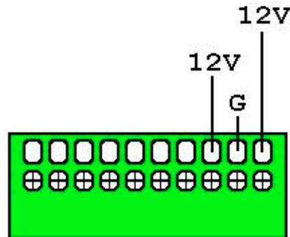
FIGURE B-2. Voltage Interface Power Connection
