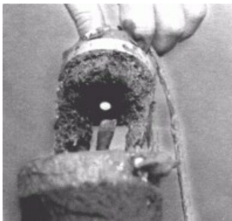
FIGURE 4-1. Preventing Bio-fouling of the CS510-L
