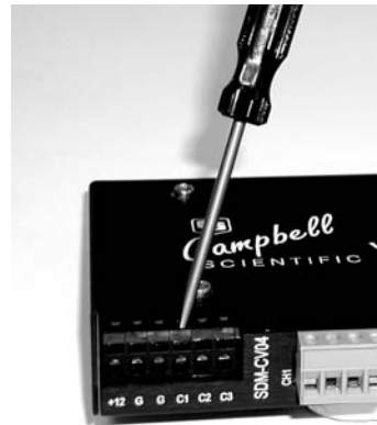
FIGURE 2-1. Use of the Spring-Loaded Terminal Blocks (Top Position)
