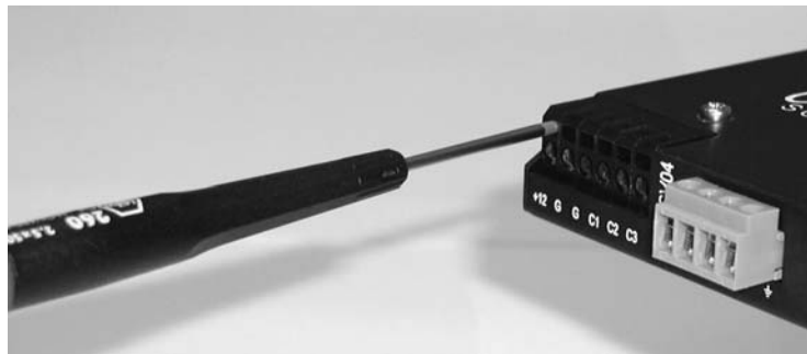
FIGURE 2-2. Use of the Spring-Loaded Terminal Blocks (Front Position)
