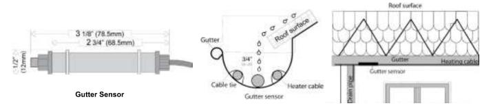
Place the sensor below the drip rim close to the down pipe to ensure that melt water will drip onto the sensor. As shown in the example above, heating conductors are also installed on the lower part of the roof surface. This keeps a sufficient area in and above the gutter free from ice and snow, thus facilitating a proper drainage of the melt water.
