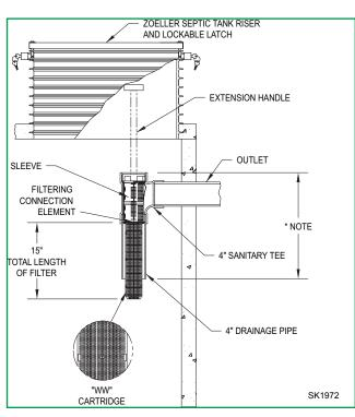
**NOTE:** State and local plumbing codes may require a specific liquid penetration. For example, 25%-45% into the liquid depth or 9" off the tank bottom.
