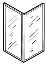
**General:** Furnish and install as shown on plans, a STYLEMATE® Double-Threshold enclosure as manufactured by E.L. Mustee & Sons, Inc. Model 36.202 with bright Chrome finished aluminum frame. Shall be double-threshold style with aluminum frame and clear tempered safety glass panel. Continuous pull handle with magnetic seal. Out-of-plumb condition up to 1" can be adjusted. Shall meet ANSI Specifications Z97.1
