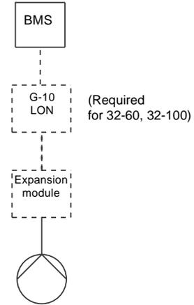
Fig. 15 Example of single-pump operation 32-60, 32-100
