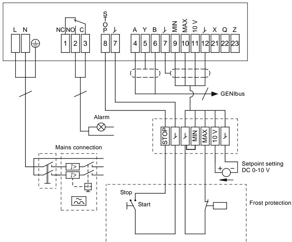
Fig. 23 Example of MAGNA pump with GENI module
