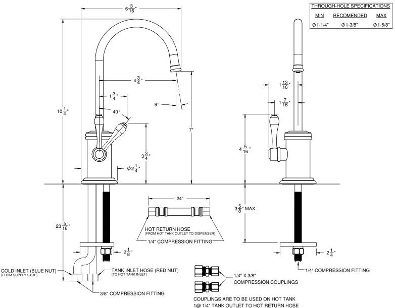
1@ 3/8" TANK INLET TO TANK INLET HOSE
