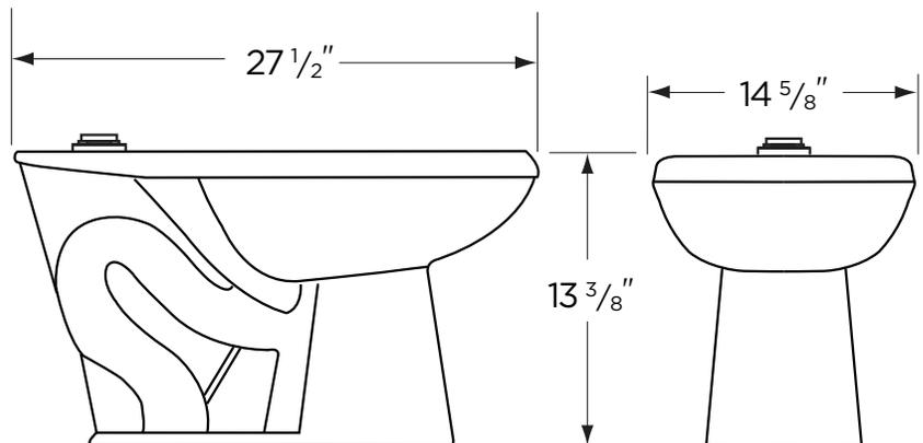
THIS FIXTURE QUALIFIES ACCORDING TO ASME TEST PROCEDURES AS A HIGH EFFICIENCY WATER CLOSET WITH AN AVERAGE CONSUMPTION OF 1.28 gpf (4.8 Lpf) OR LESS.
