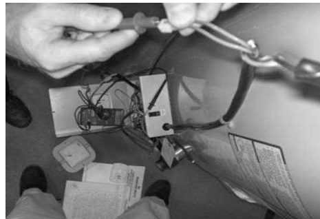
Checking continuity of upper sensor wire harness.
