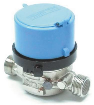
The **SJZ-K** is a single-jet meter. The operating principle which is based on water passing through the measuring chamber, causing the turbine to turn.
