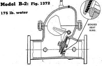
The Grinnell Backflow Prevention Device (Double Check Valve Assembly) Model B-2 is for use in water lines to prevent polluted water from entering into a potable water system.
