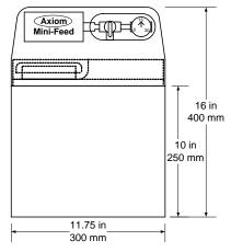
Depth - 11.75 in 300 mm Clearances - Sides and Top - 12 in 305 mm Weight When Full 60 lbs/27 kg. Discharge 1/2" FPT
