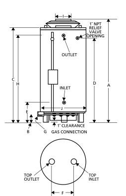
Maximum gas supply pressure (natural and propane gas): 14"w.c. Minimum gas supply pressure, natural gas: 4.5" w.c. Minimum gas supply pressure, propane gas: 11"w.c. Manifold pressure, natural gas: 3.5" w.c. Manifold pressure, propane gas: 10"w.c. Electrical requirements: 120 VAC,.7Amp, Electrical requirements with Power Venter: 120 VAC,3.0 FLAAmps
