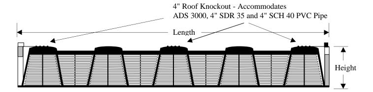
Bio 2 and Bio 3 sizes can withstand H-10 loads when installed with properly graded and compacted soils. A minimum of 12" of cover is required for H-10 loads.
