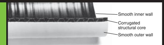
Three bonded polyethylene layers for exceptional pipe stiffness. A smooth inner wall is co-extruded with a corrugated structural core, which is then extrusion-laminated with a smooth white outer wall. This construction gives the pipe an unprecedented strength-to-weight ratio, and stiffness ratings at least double that of any competitive sewer and drain pipe.
