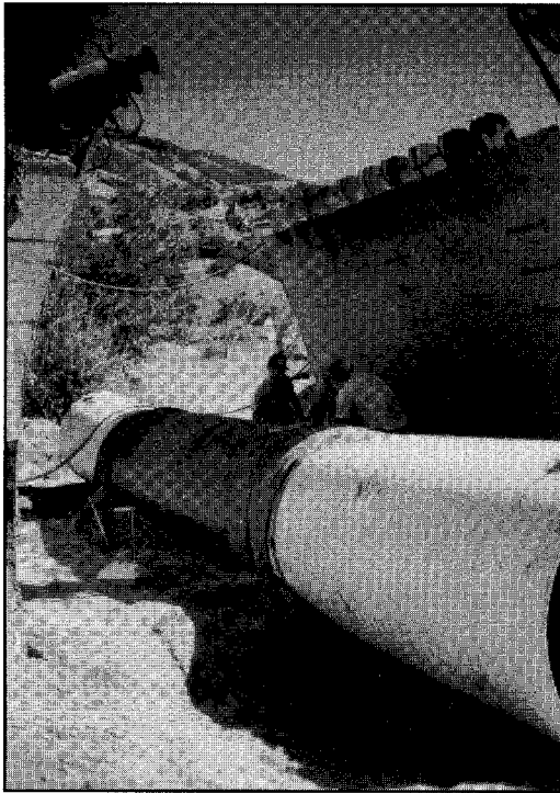
Figure 4. Test pipe (black) being placed, along with two white access pipes, in large pipe test cell at Utah State University.
