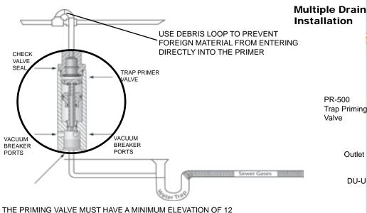
Service 1/2" Valve 12 mm 12" PR-500 Trap Priming Valve Outlet DU-U Drain Supply Line Minimum 1/2" Copper
