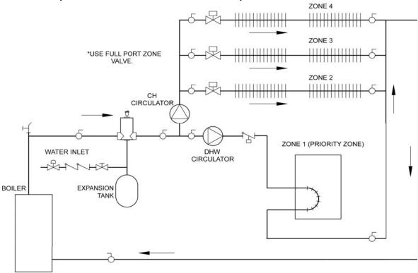
Figure 8 - Multi-zone System With Zone Valves And DHW Priority (With Zone Valve)
