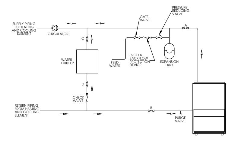
Figure 3 - Bypass Piping -Automatic Mixing Valve, See Bypass Piping Options, Page 9
