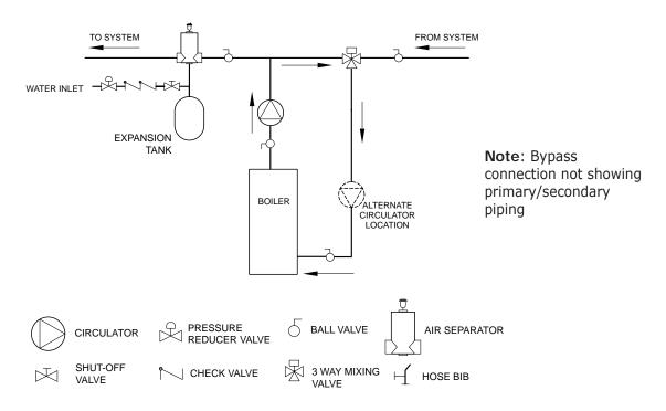
Figure 4 - Bypass Piping - Fixed Low Temp Only, See Bypass Piping Options, Page 9
