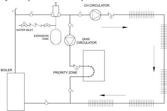
Figure 6 - Multi-Zone System with Circulators and DHW Priority
